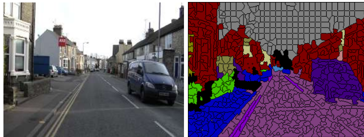
Figure 3.1.1: Semantic segmentation of an image using superpixels. The original image is shown at the left. The right image shows the superpixel-over-segmented image where each superpixel has been assigned a semantic label indicated by a color.
