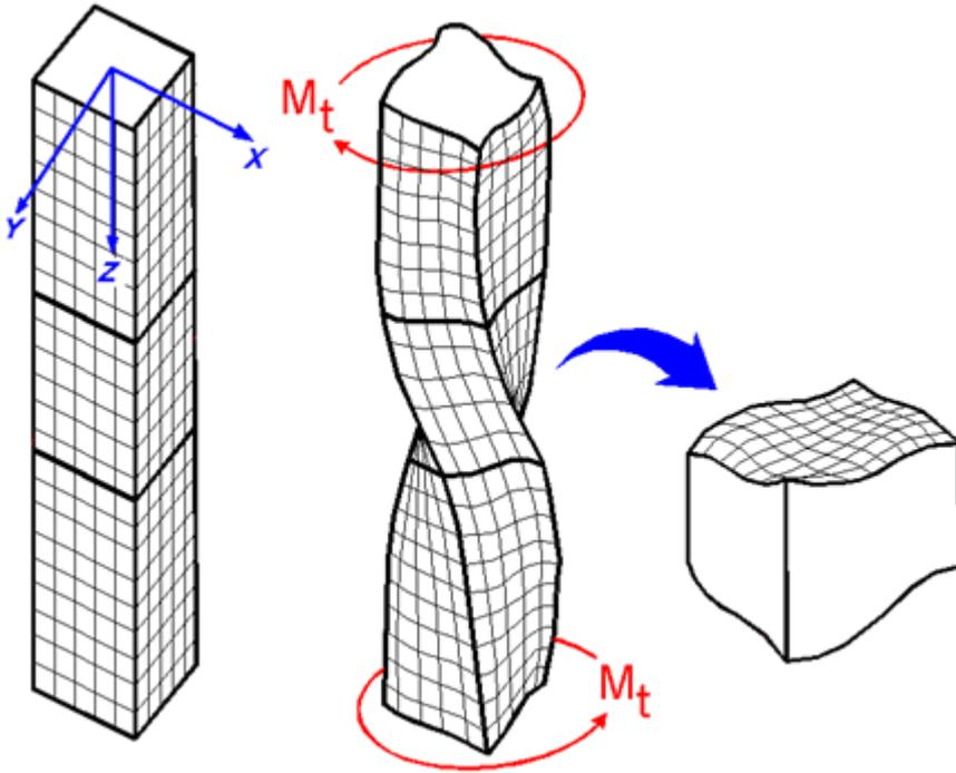
$$\frac{\partial^2 \phi}{\partial x^2} + \frac{\partial^2 \phi}{\partial y^2} = -2 G \theta$$
