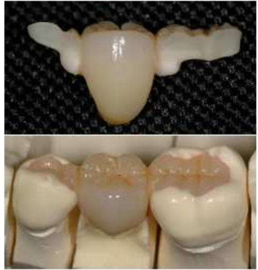
FIG. 62 This dental bridge is made from a fiber reinforced composite with braided fibers made from polyethylene. Due to the braided structure, this composite is four times tougher than a composite made from the same materials, but without the braiding (Karbhari and Strassler, 2007) (Courtesy H. Strassler, Univ. of Maryland Dental School and V. Karbhari, Univ. of Alabama, Huntsville).
